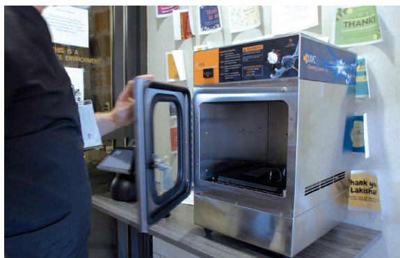
A UV cabinet is used for sanitizing smaller items such as mobile phones, laptops and eyeglasses.
